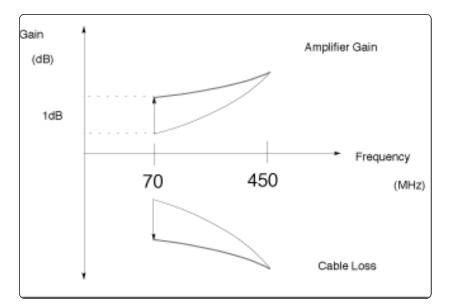
Figure 10. Cable loss and amplifier gain when tilt =1 dB
