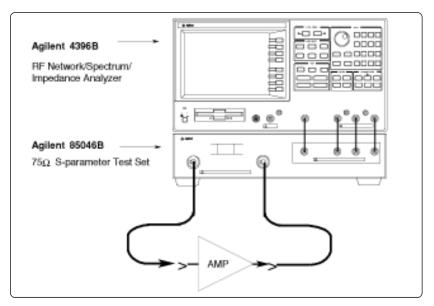
Figure 2. Example of network measurement system configuration
