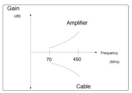
$Loss\_span(f) [dB] = Loss(f) / {Loss(450) / G(450)} + 1$
