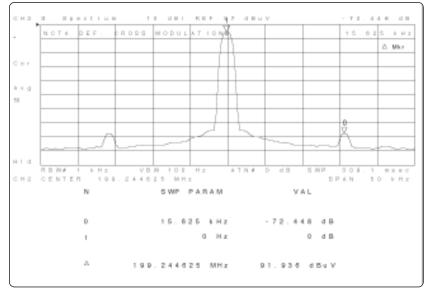
Figure 20. Example of cross modulation distortion neasurement results using the Agilent 4396B (per NCTA standard)
