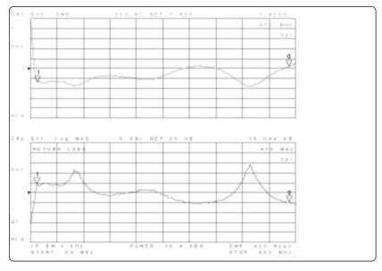
Figure 13. CATV amplifier reflection characteristic measurement results
