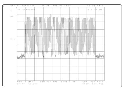
Figure 16. Carrier output from multi-channel signal generator
