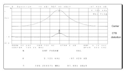
Figure 17. CTB measurement results using the Agilent 4396B
